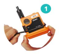
Remove the sMRT AU10 from the PFD, as per manufacturer's instructions and lift the RESTRAINER TAB up and over the ARMING SWITCH.
