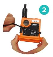
Slide the ARMING SWITCH down to the [ON] position until it clicks into place and ensure the RESTRAINER TAB is positioned in the gap above the ARMING SWITCH.
