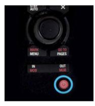
3. Press and hold the red POWER button to turn the chart plotter
