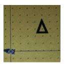
1. The screen displays a black triangle when AIS data is first received from a locator beacon.
