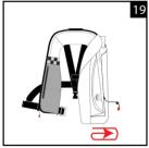
Fold the left side bladder lobe (as worn) twice at the outer edge so that the inflator sits on the back.
