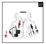
Fold the bottom part of the right side bladder lobe (as worn) back towards the lower edge of the cover; tucking the surplus underneath. Ensure the beacon is positioned directly above the antenna pouch
