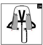
Clip the crutch strap into the buckles on the centre back strap and left front belt
