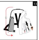
Then pull the zip slider all the way back down again to the bottom centre front. The zip should now be completely closed on this side and the bladder, beacon and antenna securely inside the cover.
