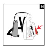
Attach the grab/lifting strap onto the velcro on the bladder.
