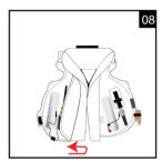
Fold the right side bladder lobe (as worn) at the centre front edge once to the outer edge.
