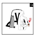
Fold the bottom part of the left side bladder lobe (as worn) away from the lower edge of the cover.
