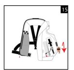
Fold the bottom part of the left side of the bladder lobe (as worn) back towards the lower edge of the cover; tucking the surplus underneath.
