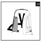
Position the inflator pull cord and handle out of the back slot in the cover ensuring that it hangs down freely at the back.
