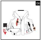
Fold the bottom part of the right side bladder lobe (as worn) away from the lower edge of the cover.
