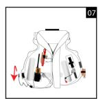
Fold the bottom part of the right side of the bladder lobe (as worn) back towards the lower edge of the cover; tucking the surplus underneath.
