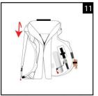
Fold the top corner outer edge down and in towards the centre front.
