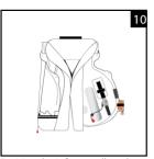
Position the inflator pull cord and handle out of the back slot in the cover ensuring that it hangs down freely at the back.
