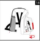
Fold the left side bladder lobe (as worn) at the outer edge so that the buddyline is tucked away to the back.
